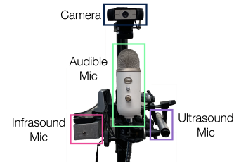
Figure 2: An image of the wide-band audio capture rig, consisting of infrasound, audible, and ultrasonic microphones, along with a camera. The set-up is used to capture sounds from 127 different objects and devices commonly found in residential homes and commercial buildings. The data is used to determine which frequency components are most predictive of object and device usage.
