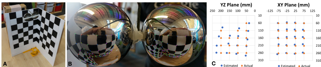
Figure 8. A) Orthogonal checkerboard setup, with headset mounted at top. B) View of checkerboard from headset with intersections denoted. C) 3D error in YZ and XY Planes.
