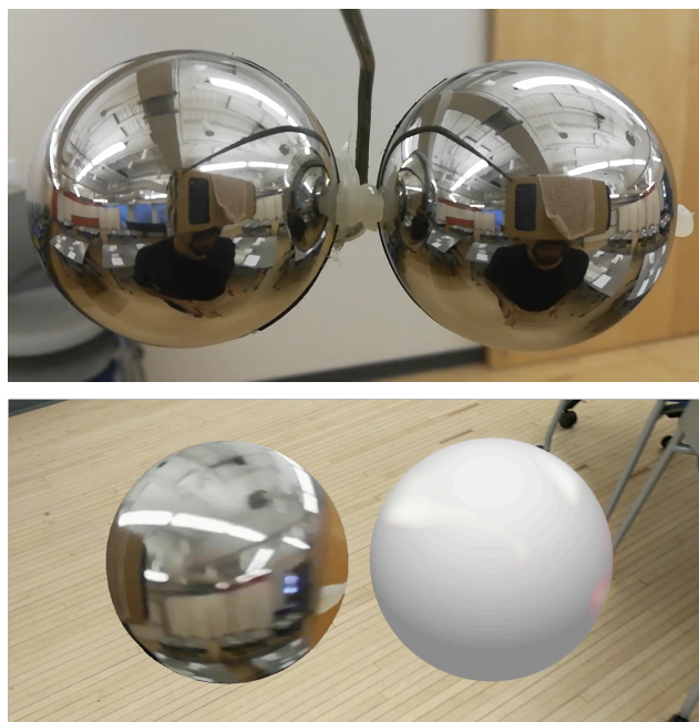
Figure 7. View from front-facing camera (top) used to create a realistic environment map on two virtual spheres (bottom; specular and diffused reflection).
