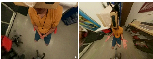
Figure 3. Synthetic camera views MeCap uses to capture the hands (left) and body pose (right).
