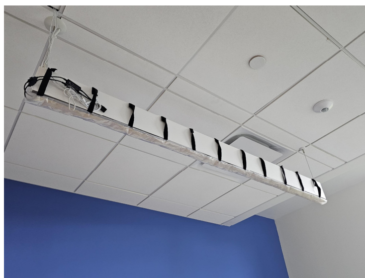
Figure 2. Custom Light setup. LED lights were attached to the bottom of the room's existing light fixture (direct light) and were placed on top (indirect light).
