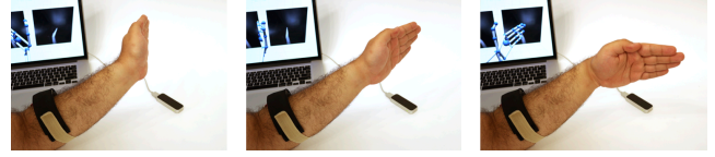
Figure 17. Our wrist angle task used a Leap Motion controller to provide ground truth. Here a participant sweeps their hand from left to right (with all intermediate angles recorded).
