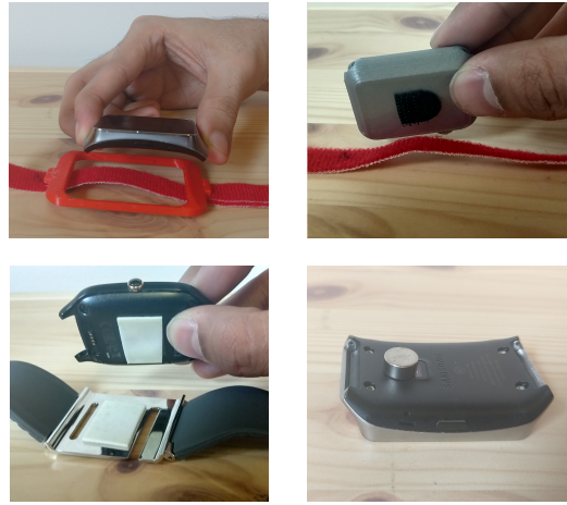
Fig. 3. Prototypes of different detachability mechanisms. Press fit (top-left); Velcro (top-right); 2-sided tape (bottom-left); and magnets (bottom-right)
