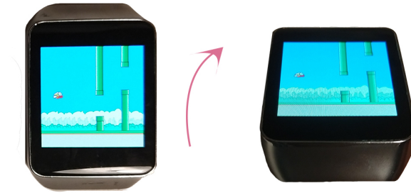
Fig. 5. The rotation of the watch (accelerometer) is used as an input to control the character in a game
